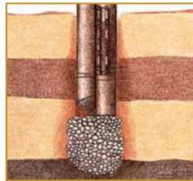
The stones are introduced via a tremie pipe along the vibroflot and the aid of pressurized air.
