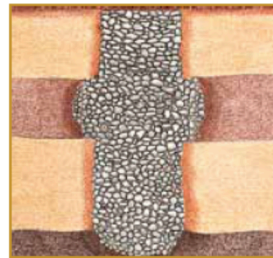
The vibroflot is frequently moved up and down in order to form and compact a column. Thereby, the surrounding ground is horizontally compressed and improved. The column is able to support high vertical loads.
