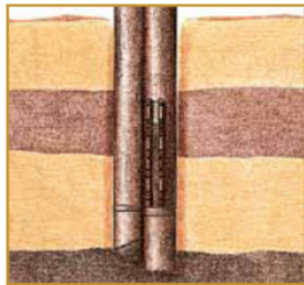
The vibroflot penetrates with the help of vibration and air flushing. (sometimes a minimal water lubrication is helpful to overcome high friction from the soils)
