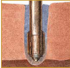
The vibroflot penetrates and 'washes' the hole in preparation for the stone transport within the hole.
